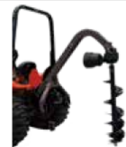
POST HOLE DIGGER
